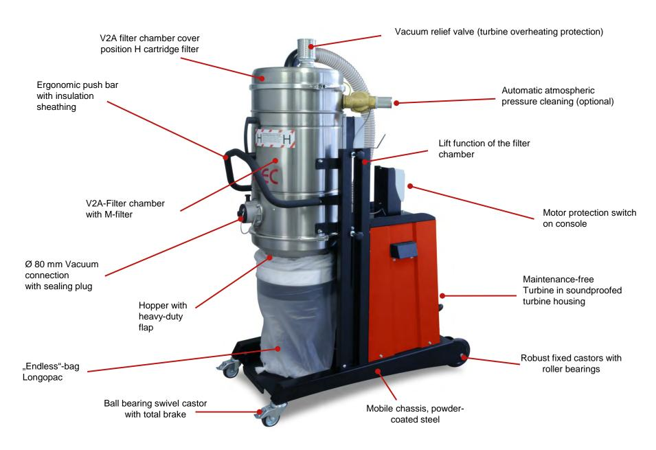
Super-silent industrial vacuum cleaner for vacuuming all dry dusts - from coarse dirt to micro particles (µm)
