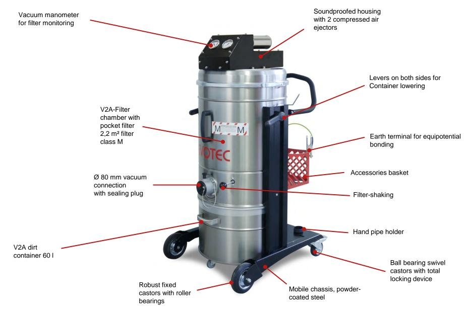
High quality standards– well designed, powerful compressedair ejectors with silencer for the secure usage even in explosive areas (Zones 1/2 and 21/22).
