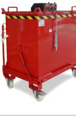
Container with hinged floor 1000 liters With Ø 80 connections For pre-separation of solids (e.g. peat, earth, sand, etc.) Tension springs dampen the bottom flap during the emptying process Automatic closing of the bottom flap during settling Unlocking by cable from the forklift seat
